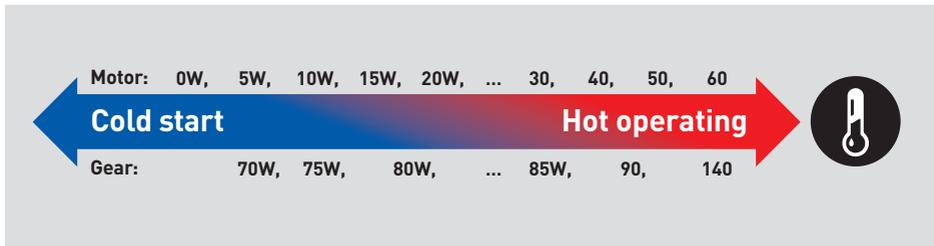
The minimum low temperature at which a motor/gear oil can be used depends on the possible borderline pumping temperature or the low-temperature viscosity.
